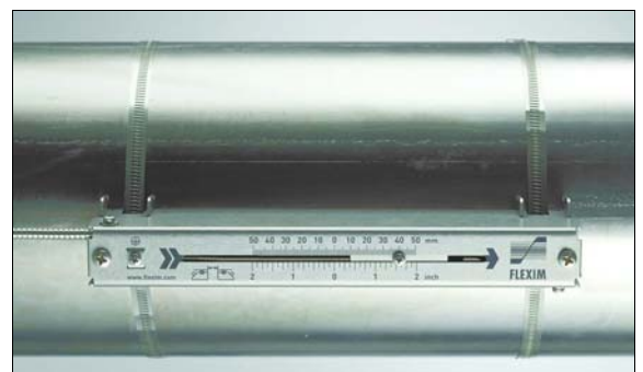
Measurement with transducers mounted by Variofix L
