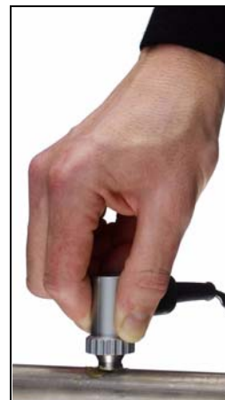
Wall thickness measurement
